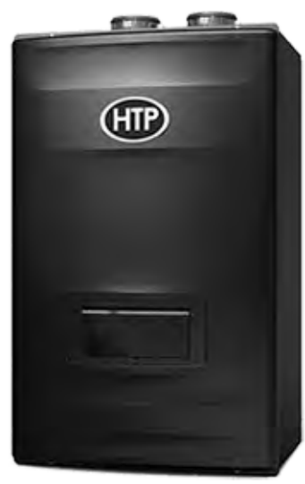
Name (Brand): Wall-mounted Boiler (HTP) Size: TBD by Craig Tarr Location: Mechanical Quantity: 1 Details: 316 L stainless steel fire tube heat exchanger with a 96% AFUE rating; Energy Star approved; Adaptable to fit installation requirements
