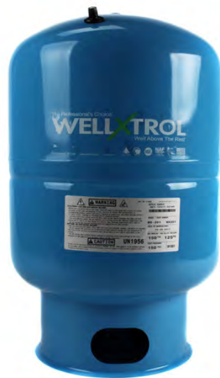
Name (Brand): Expansion Tank for Well (AMTROL) Size: TBD by Craig Tarr Location: Mechanical Quantity: 1 Details: Strongest tank design featuring deep drawn steel and multi-dome construction; Thickest diaphragm made of heavy duty butyl;
