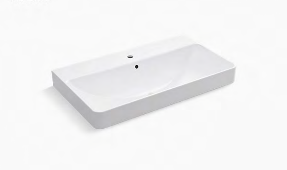
Name (Brand): Trough Sink (KOHLER) Size: 36" W x 21" D x 6" H Location: Bathroom Quantity: 1 Details: Meets ADA requirements; Vitreous china coating; Above counter sink basin with contemporary design; Convenient overflow placement
