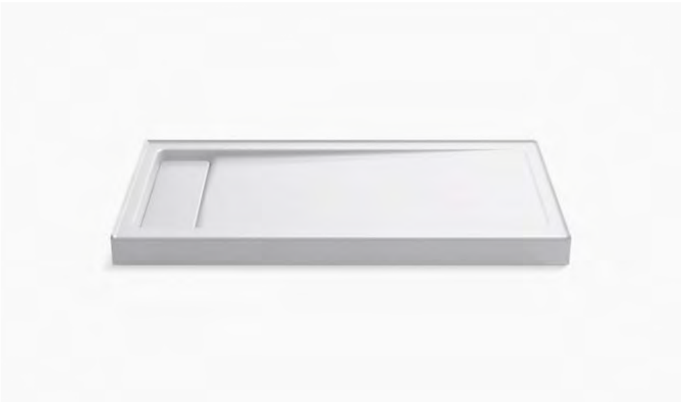
Name (Brand): Shower Basin (KOHLER) Size: 60" W x 32" D x 4" H Location: Bathroom Quantity: 2 Details: Safeguard® slip-resistant finish for added safety; Cast iron with Safeguard® finish; Left centered drain with removable drain cover
