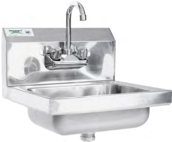
Name (Brand): Handwashing Sink (REGENCY) Size: 17" W x 15" D Location: Kitchen Quantity: 1 Details: Made of 20-gauge type 304 stainless steel; 8" high backsplash; Durable construction; Includes mounting bracket
